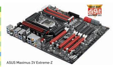
Apart from the SSD, the board is quite similar to the Z68AP-D3. The build quality of the board is quite good with sturdy heatsinks. The PCIe slots can be used for SLI as well as CrossFire, but one of them runs at x8 speed.
